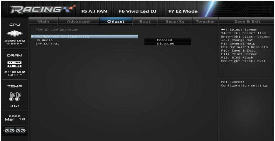
The screenshot shows the BIOS 'PCH-IO Configuration' menu. The 'Chipset' tab is selected. The 'HD Audio' option is set to 'Enabled' and 'ErP Control' is set to 'Disabled'. The left sidebar shows system information: CPU at 2.609 MHz, DRAM at 2.140 MHz, and temperature at 36°C. The top navigation bar includes 'F5 A.I FAN', 'F6 Vivid Led DJ', and 'F7 EZ Mode'. The right sidebar contains a list of BIOS navigation keys and a 'PCI Express Configuration settings' link.
